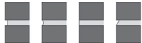
Raked Joint Ironed/Rolled Joint Flush Joint Struck Joint
