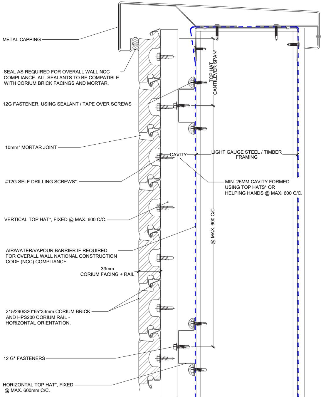
Fig 10: Typical Slab Edge – CORIUM Section Detail
