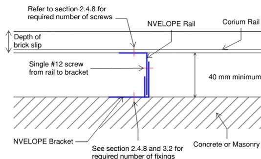
If the stud set out does not align with the vertical support set out, horizontal top hats will have to be first fixed to the studs, and then vertical top hats (of at least 25 mm height) placed on top, connecting to the CORIUM rail. If this method is used, precautions will need to be made for the effect that the weight of the CORIUM system has in compromising the performance of the horizontal top hat. Please consult with the manufacturer of the horizontal top hat for guidance.
