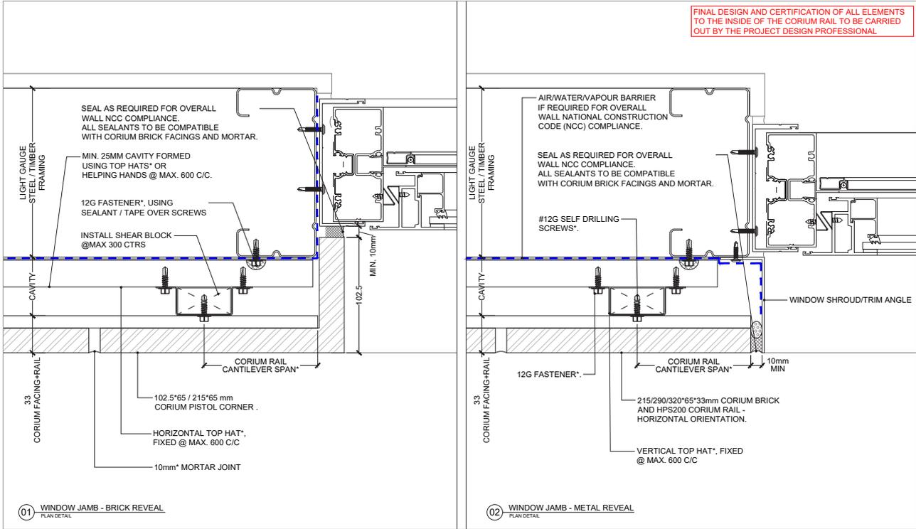
Fig 26: CORIUM door jamb detail. The detail for steel/timber framed substrates will be near identical except that the vertical supports must be selected accordingly in accordance with section 2.4.5.
