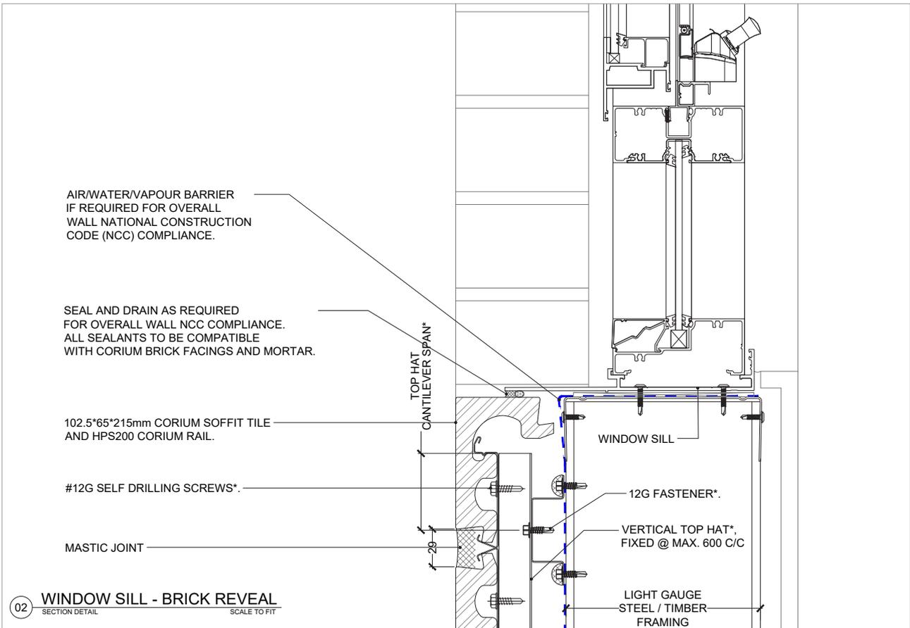
Fig 15: Window Metal Reveal – CORIUM Section Detail
