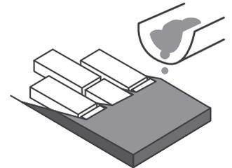
When the InBrick panel is erected, the VersaLiner® is stripped from the face and the panels are cleaned. The end result is an InBrick concrete precast panel with an InBrick cast façade.
