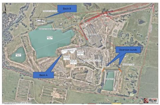
Figure 1 – Surface run off water diversion design
