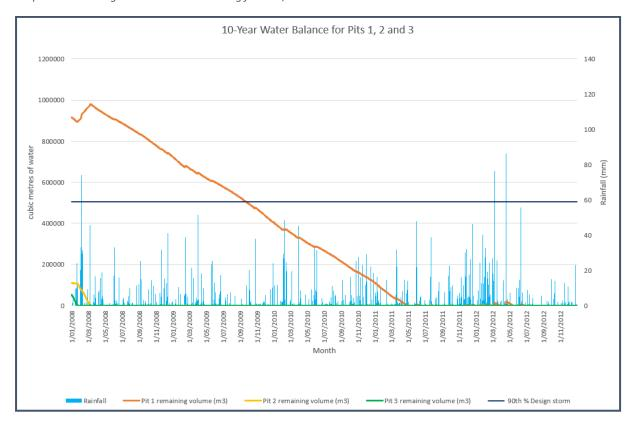
As can be seen from Graph 6: Dewatering Water Balance Modelling for Pit 1,Pit 2 and Pit 3, dewatering of Pits 2 and 3 will take several months each and Pit 1 will take approximately three years based on rainfall for the critical period between 2008 and 2017.
