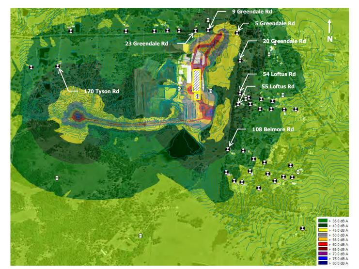
Figure 6-6 Predicted Noise Levels for Stage 3 Campaign Cell I Operations – Calm Meteorological Conditions (Mitigated), LAeg, 15min
