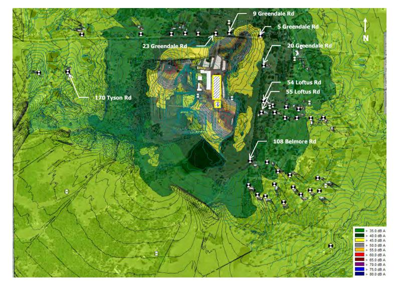
Figure 6-5 Predicted Noise Levels for Stage 2 Campaign – Calm Meteorological Conditions (Mitigated), L<sub>Aeq,15min</sub>
