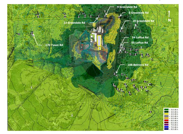
Figure 6-4 Predicted Noise Levels for Stage 1 Campaign – Calm Meteorological Conditions (Mitigated), L<sub>Aeq,15min</sub>
