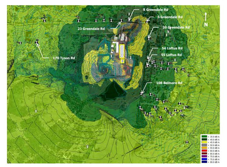
Figure 6-7 Predicted Noise Levels for Stage 3 Campaign Cell G Operations – Calm Meteorological Conditions (Mitigated), LAeq, 15min
