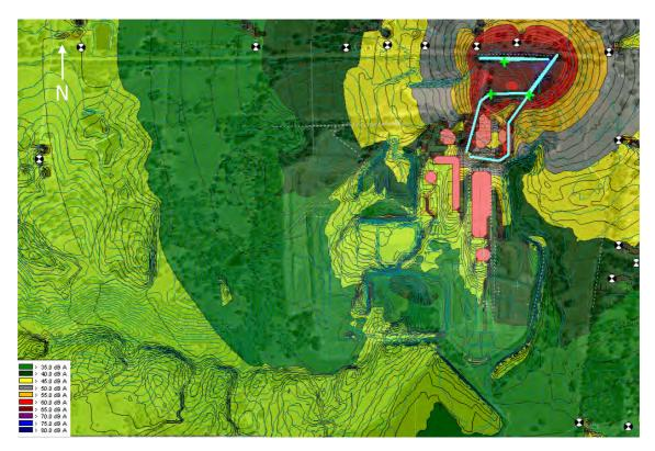
Figure 8-2 Noise Contours for Construction Scenario A - Road Works
