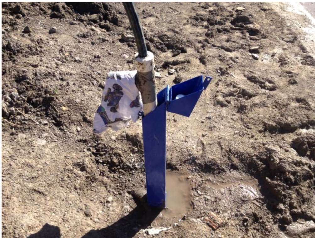
Figure 7: PVC T-piece and air line for well development by airlifting
