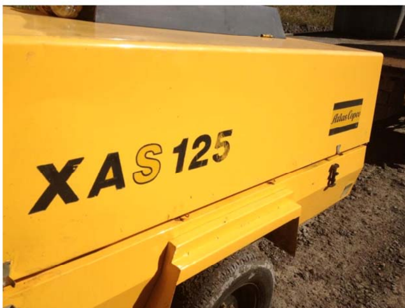
Figure 6: Portable air compressor used for airlifting well development
