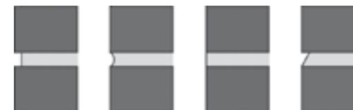
**Raked Joint**   **Ironed/Rolled Joint**   **Flush Joint**   **Struck Joint**
